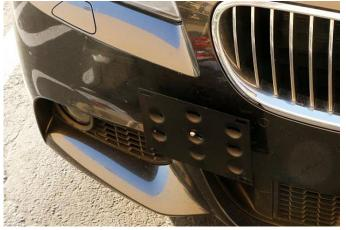
Step 3: Then screw the license plate onto the tow hook plate bracket.
