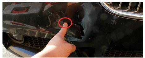
Step 2: Insert license plate mount stick. Make sure it's perpendicular to the opening. Slowly turn the stick clockwise until it catches on. To tighten the stick, use a wrench. Once the tow stick is fully tightened in, then it is time to mount the license plate bracket. You can use the metal flat washer and the spring washer included in the package to "sandwich" the bracket. This will increase friction to prevent spinning. Do not use power tools! Instead, use a regular Phillips screwdriver.
